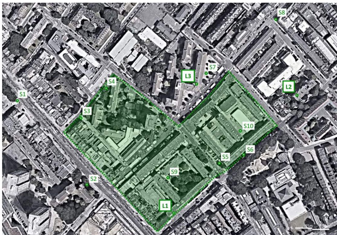
Figure 7-3: Aerial image of the Application site showing noise survey locations (Google Maps).
